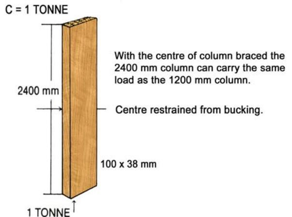
Where this rigid support is applied to a web member, it is called a web tie, which is used in conjunction with bracing. (See Figure 5A)
