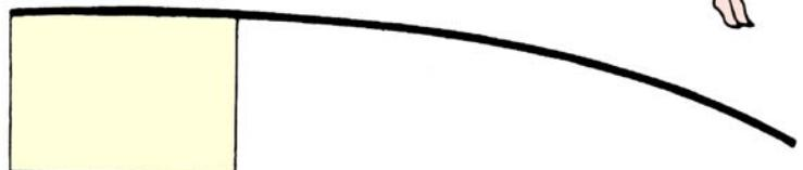
**Bending** force, or more correctly bending moment, is the result of a force applied to a cantilever, for example: a diving board, or to a simple beam.
