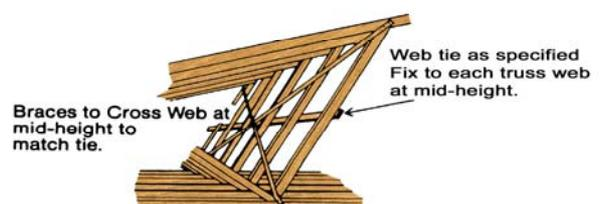
Battens with bracing from the rigid supports are needed to restrain the truss chords from buckling sideways. (See Figure 5b).
