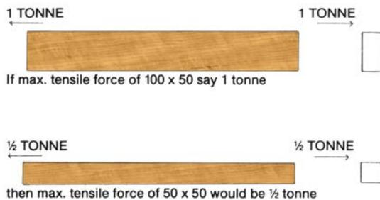
The example shows that if the cross-sectional area of a member is doubled, the ability of that member to restrain the tension forces is also doubled.
