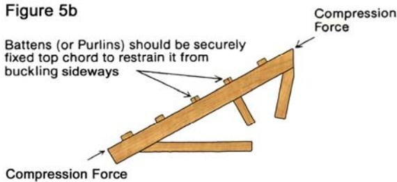
The strength of a column is also dependent on the cross-sectional shape of a column. The squarer or more symmetrical the shape, the stronger the
