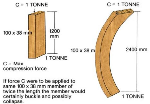
However, if we rigidly support the 2400 mm long column in the previous example at the centre, it would then be capable of withstanding the one tonne force.
