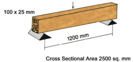
Deeper sections having the same cross sectional area are stronger in bending.
