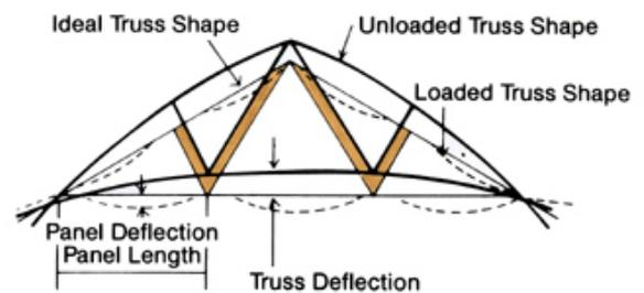
Exaggerated long term truss deformation under distributed top and bottom chord loads.
