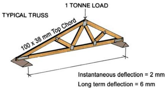
From these examples, it can be readily appreciated that timber trusses are very effective structural components.
